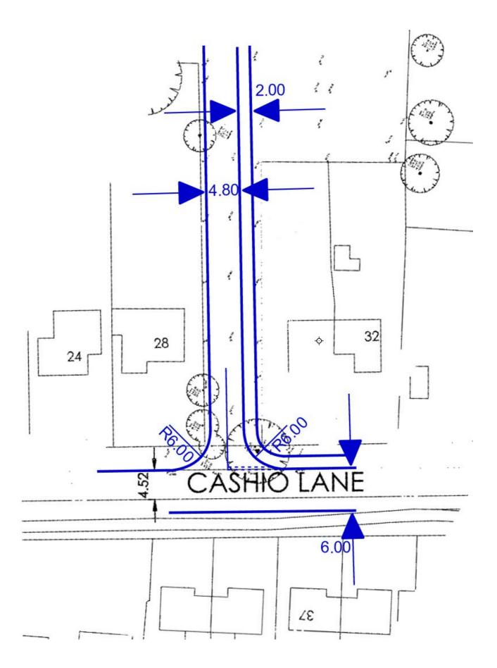
Our illustration shows a 2m footway, sufficient for two wheelchairs to pass, rather than the 1.8m footway proposed by the applicant.
